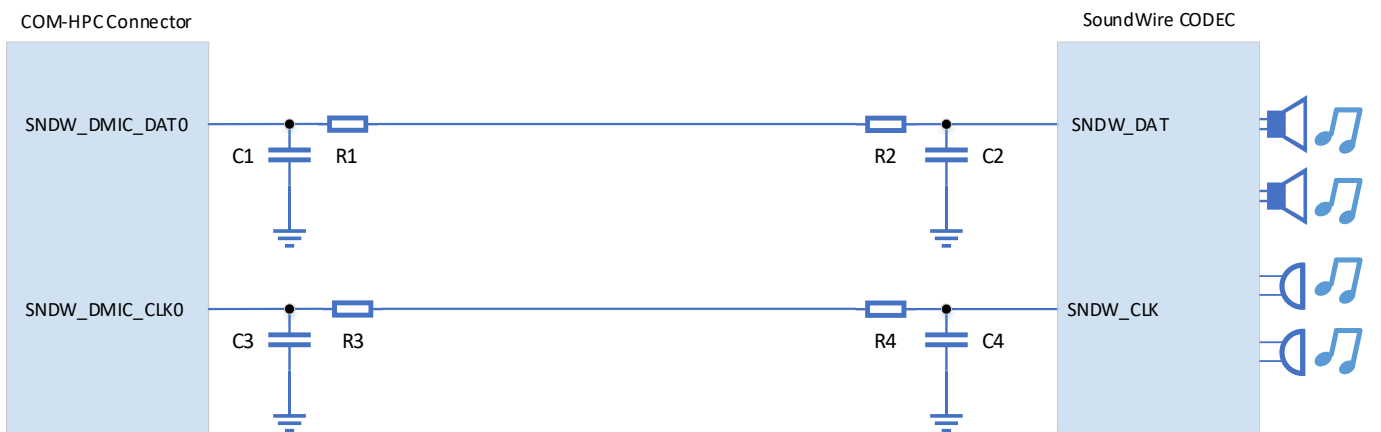
Figure 47: MIPI SoundWire Point to Point Connection With SI Components
